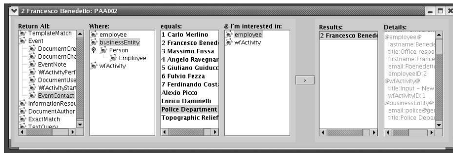
Fig. 2. Query creation GUI. Query on the picture can be read as follows: Return All EventContacts where BusinessEntity (contact contacted) is Police Department and I am interested in the employee, which made the contacts. Note that ontological elements adopt tree structure from inheritance of ontology elements.
